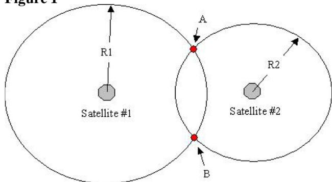
With two satellites tracking, they know that the receiver (you) are either at Point A or Point B.
